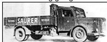
III. 132: The Saurer BT 4500 with a gas generator. A Saurer truck is supposed to have been used for mass murder at the Kulmhof/Chelmno camp – yet not by using generator gas, but allegedly its exhaust gas! (Spielberger 1976, pp. 207, 213)
