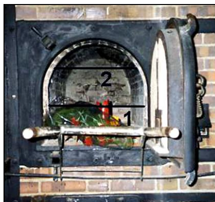
Ill. 204: Topf coke-fired double-muffle furnace Auschwitz type (here in Mauthausen). The door – 60 cm wide and high – and muffle sizes are the same as those for the Birkenau furnaces. Corpse stretcher lying on rollers. The two horizontal lines represent the height of two superimposed normal corpses resting on the muffle grid. They would be even higher while resting on the stretcher. (Mattogno 2015a, Doc. 46)
