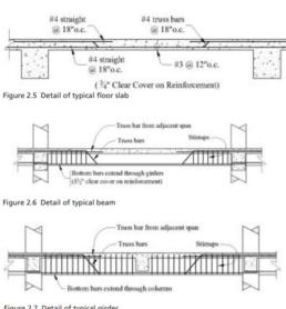
Figure 2.7 Detail of typical girder
