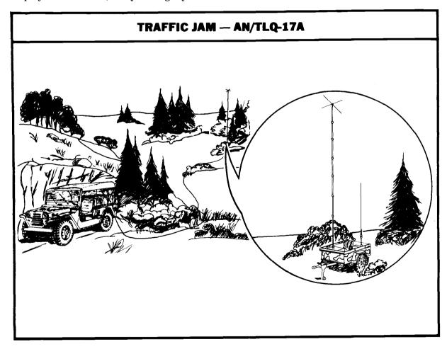
The HF band-1 antenna can be mounted in the M-416 trailer, as shown above, or dismounted and set upon more favorable terrain. The VHF band-2 whip antenna can also be trailer-mounted, as shown above. However, it is usually mounted on the rear of the M-151A to facilitate rapid set-up and tear-down time.
