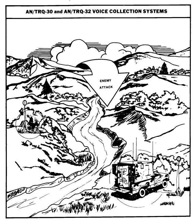
These systems have similar capabilities and limitations. They are capable of intercepting both HF and VHF single channel voice and manual Morse communications facilities supporting enemy first-echelon units.
