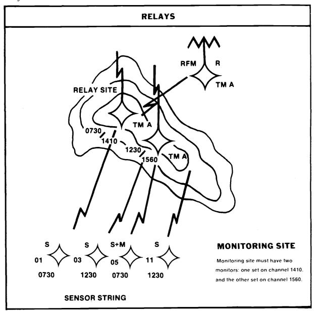
The timeliness and accuracy of sensor-derived data make REMS an excellent target acquisition resource. The REMS team emplaces sensors near predesignated target areas and reports activations to the FIST. Properly employed, REMS can indicate the type, size, number, direction of movement, and speed of the target.
