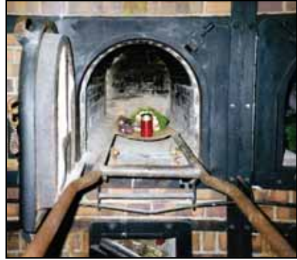
Ill. 124: Typical corpse stretcher, here from a cremation oven of the Mauthausen camp. (Mattogno 2010a, doc. 44)
