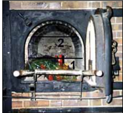
Ill. 122: Topf coke-fired double-muffle oven Auschwitz type (here in Mauthausen). The doors are the same as those for the Birkenau ovens. Corpse stretcher lying on rollers. The two horizontal lines represent the height of two superimposed normal corpses resting on the muffle grid. They would be even higher while resting on the stretcher. (Mattogno 2010a, doc. 46)
