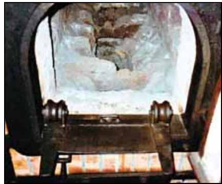
III. 121: Topf triple-muffle coke-fired oven type Birkenau (here in Buchenwald). Rollers for introducing corpses on stretcher or coffin cart in position for operation. (Mattogno 2010a, doc. 40)
