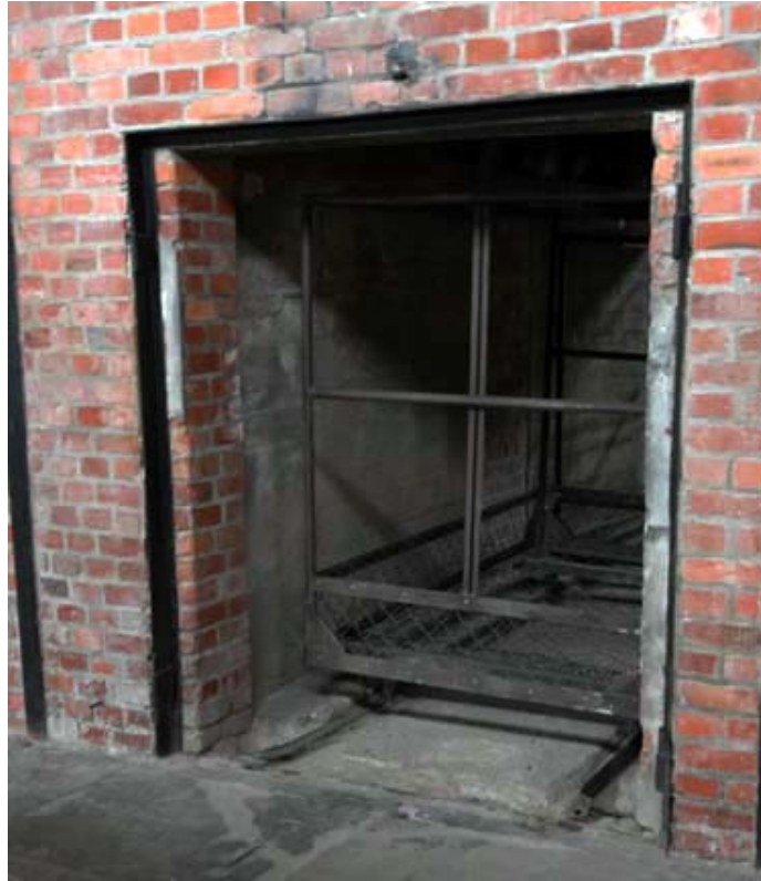
“Hot Air oven in the Central Sauna, used for killing lice in clothing”
