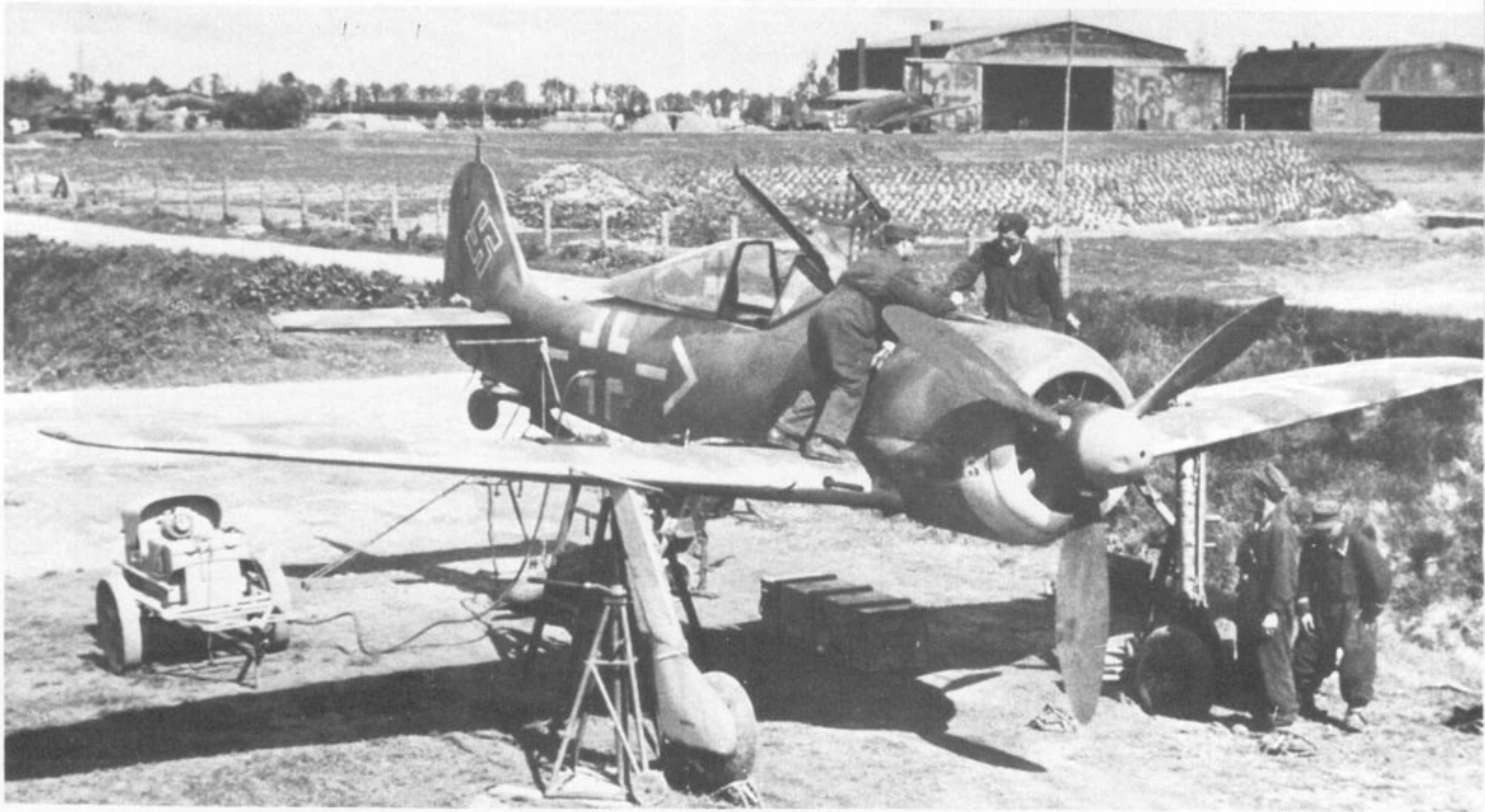
Maintenance personnel seen adjusting the internal guns of an Fw 190 in Dorpat.
