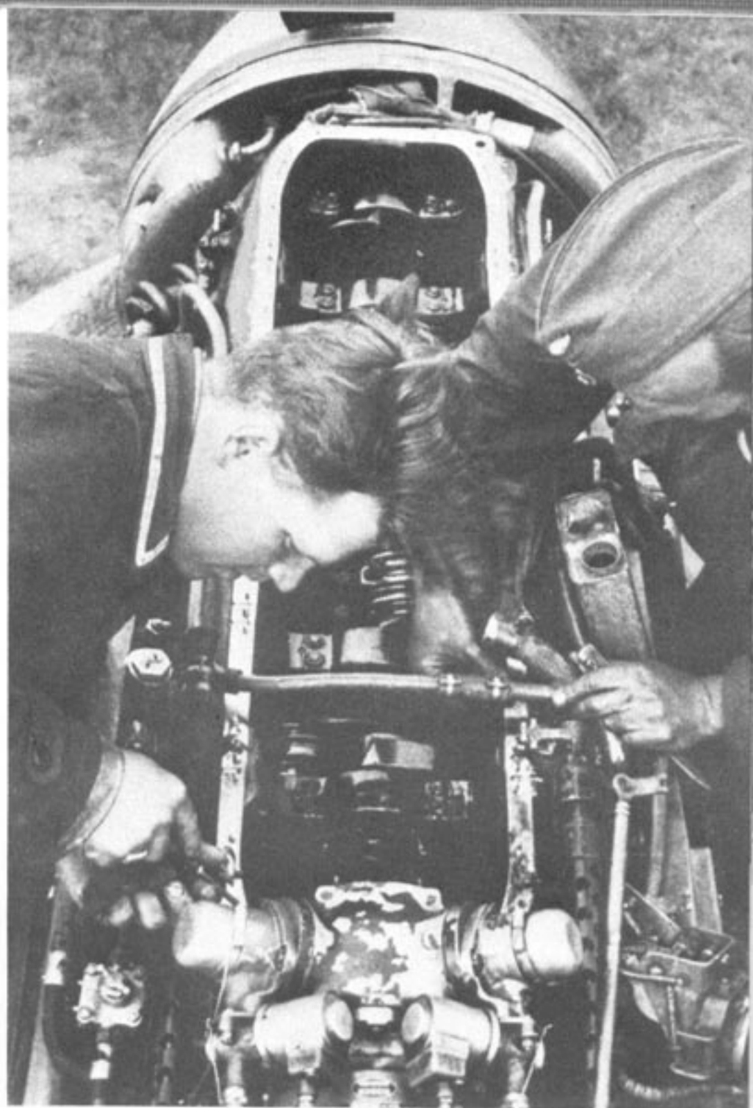
View from above showing the 12-cylinder Daimler-Benz DB 601 engine of an Bf 109 – the daily workplace for the engine mechanics.
