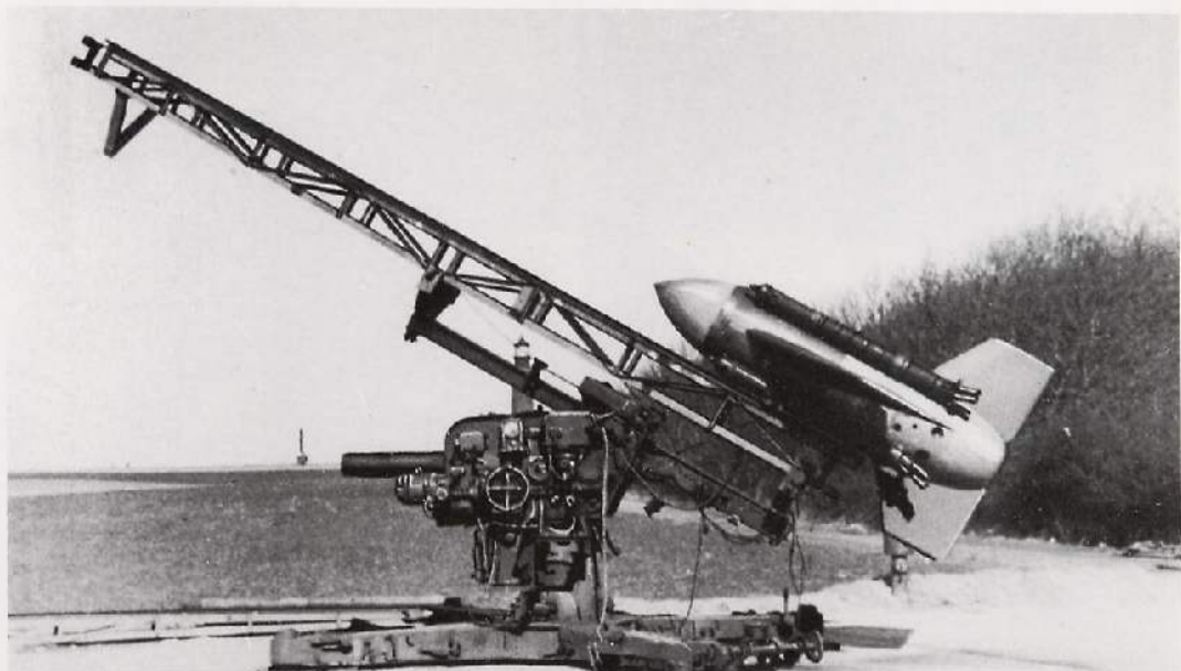
Enzian on an modified launcher, based on the 8,8 cm Flak, ready for series production.
