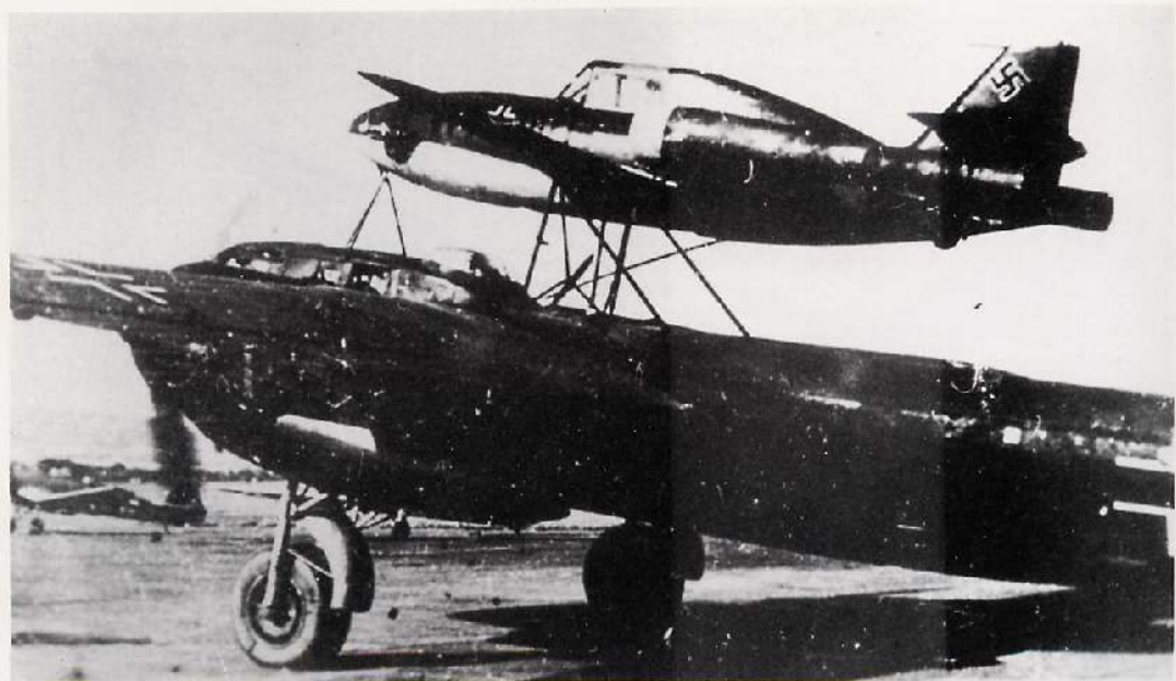
Me 328 B0/B1 on top of a Dornier Do 217 E (JT+FL) during initial flight tests.
